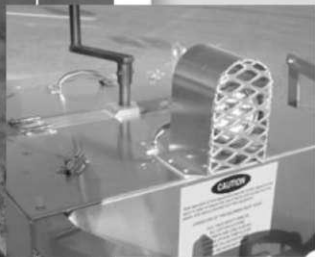
MANUALLY OPERATED AGITATOR AND MATERIAL TEMPERATURE INDICATOR
